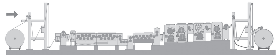
Figure 9: Chain Mercerizing Machine
